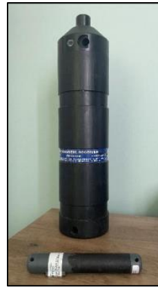
Left: A VR2Tx acoustic receiver and V16 acoustic transmitter. Right: Receivers are tethered to a marked fishing buoy and deployed from May through November with a mooring anchor.
