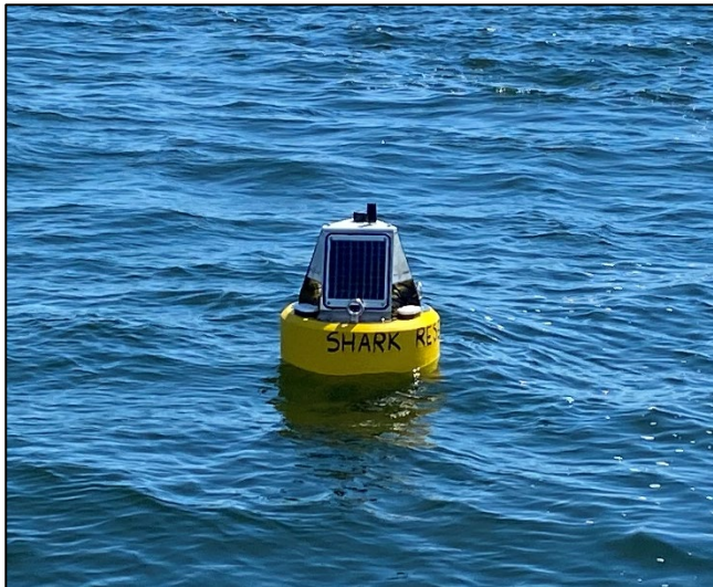
Above: The top of a real-time acoustic telemetry buoy system. The pyramidal structures atop the buoy are solar panels.
