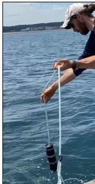
Above left: Picture of an acoustic receiver and acoustic transmitter. Above right: Deploying an acoustic receiver into the Gulf of Maine. Receivers are tethered to a marked fishing buoy.
