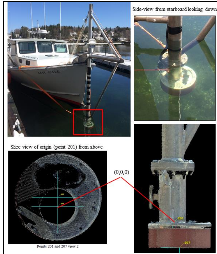
Figure 7 – Amy Gale origin (point 201 in RGB images) for vessel reference frame(s); origin is center point within the base of the pole (center point of base within internally-mounted motion reference unit (MRU) point 201 in images above)
