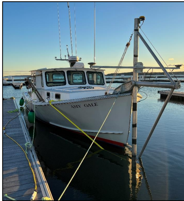
Figure 5 – F/V Amy Gale shown with pole-mounted dual GPS antennas, Fugro AD-341 antenna, Kongsberg EM2040C multibeam sonar (not visible), MRU (not visible), and surface sound speed probe (not visible) in acquisition mode.
