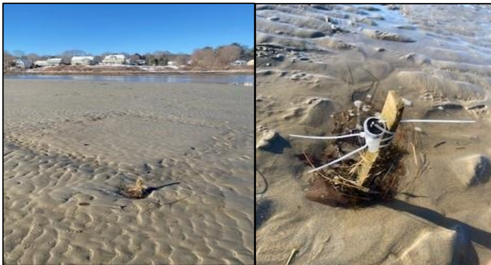
Figure 13. HOBO temperature logger on a wooden stake near a seeded plot after netting removal (left). HOBO logger on a wooden stake during a routine check of the site (right).
