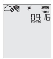
Once **READY** disappears, release the button within two seconds. **STARTING** will now disappear, and the **REC**• symbol will be shown. The VFC400-WiFi now records temperature data.
