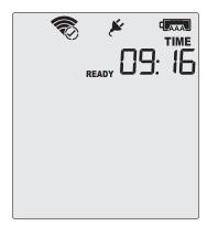
After successful completion of the wireless network test, the Wizard establishes a connection between the VFC400-WiFi and the  $LogTag^{\circledR}$  Online cloud server. When completed successfully, the screen on the right shows.
