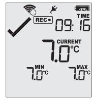
Once the VFC400-WiFi has successfully connected to the wireless network (the WLAN symbol shows a tick) it will attempt to connect to the LogTag<sup>®</sup> Online cloud server (Cloud symbol shows an empty circle).
