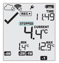
Keep holding the button until the **REC**• symbol disappears, then release the button within 2 seconds.
