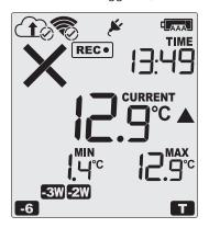
Each alarm trigger condition consists of a threshold temperature value, an activation type (which can be instant, consecutive or accumulative<sup>1</sup>) and a delay time, if it is not an instant alarm.
