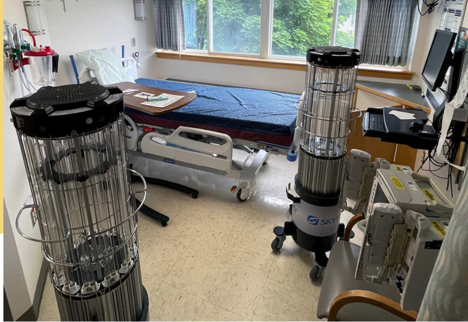
UV germicidal disinfection lights in a patient room. Photo courtesy of Northern Light AR Gould Hospital.
