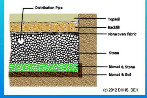
Anaerobic organisms living in the biomat digest suspended organic matter contained in the effluent before it reaches the soil, where digestion of dissolved components occurs by aerobic or facultative bacteria.
