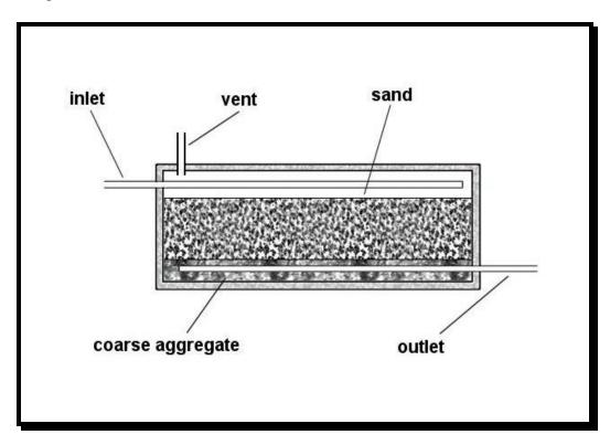
Figure 22. Cross section of under-drained sand filter.
