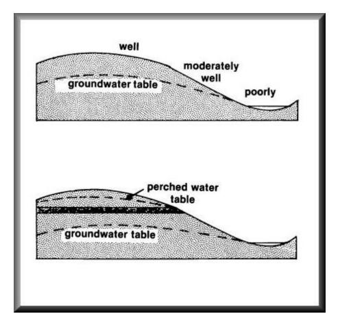
Figure 51. Soil drainage and groundwater table
