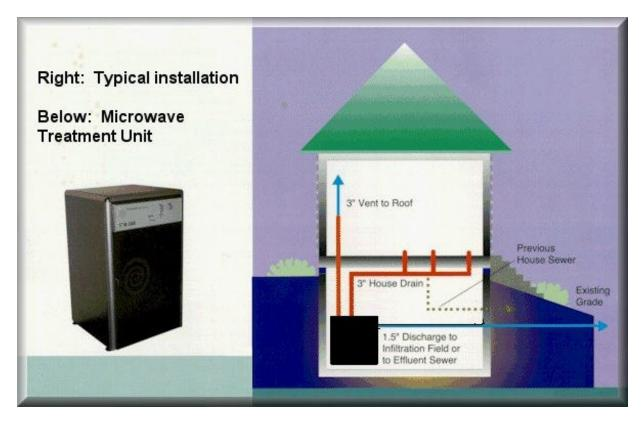
Figure 31. Typical microwave residential installation.
