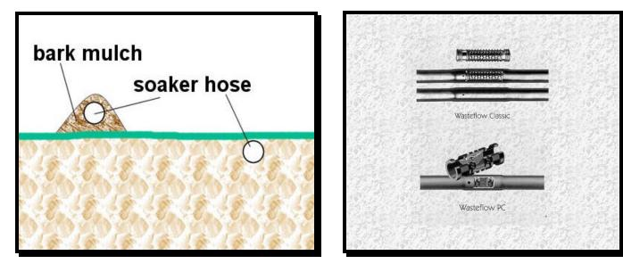
Figure 19. Porous soaker hose drip irrigation system.
