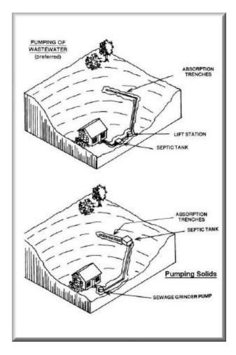
Figure 32. Effluent and sewage lift station design layouts
