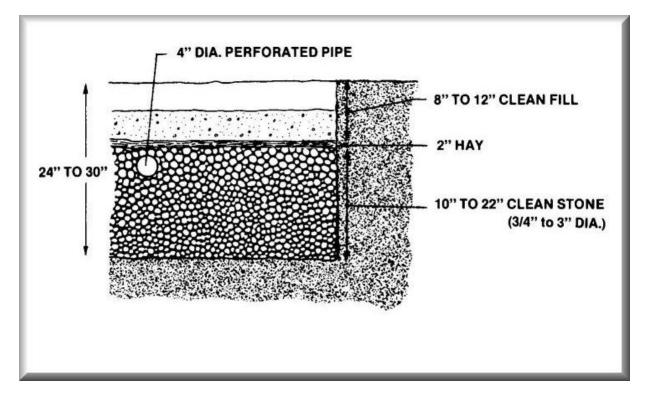
Figure 4. Cross section of disposal bed
