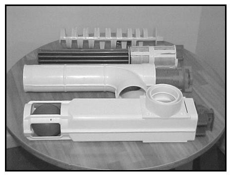
Figure 24. Residential septic tank outlet filters.
