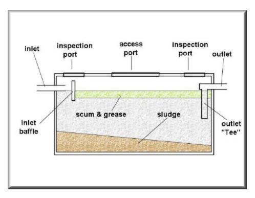
Figure 2. Cross-section of a typical septic tank.
