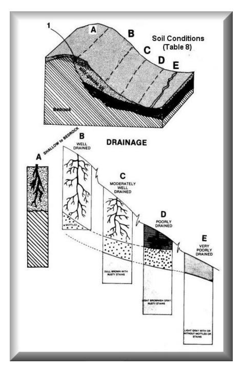
Figure 54. Natural drainage classes of soils and subsurface wastewater disposal classifications
