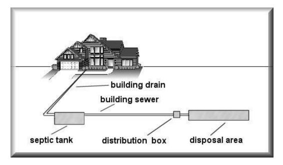
Figure 1. Essential features of a disposal system.
