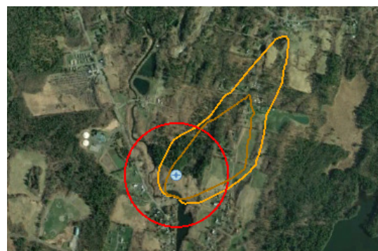
Image depicting wellhead protection area: 1000' buffer zone (red), 200-day travel zone (brown), and 2,500-day travel zone (orange).
