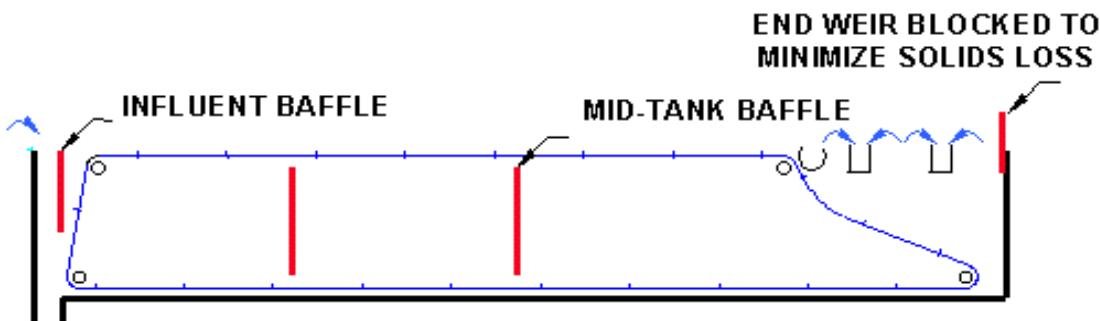
**RECTANGULAR CLARIFIER WITH TWO MID-TANK BAFFLES
