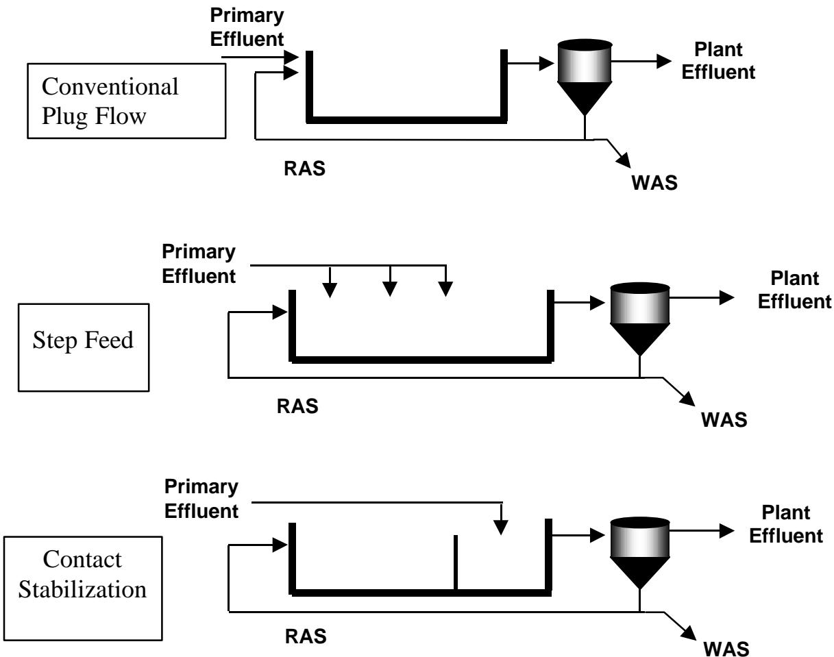
Figure 2.8 Activated Sludge Operating Modes
