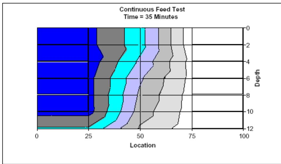
Figure 2.8 Continuous Feed Dye Test at 35 minutes
