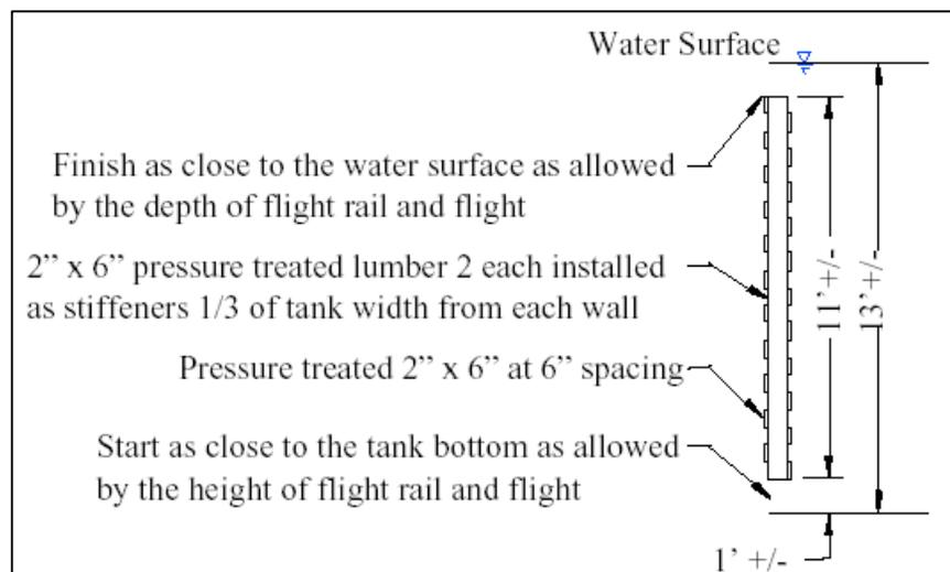
Figure 2.10 Typical Wooden Baffle Construction
