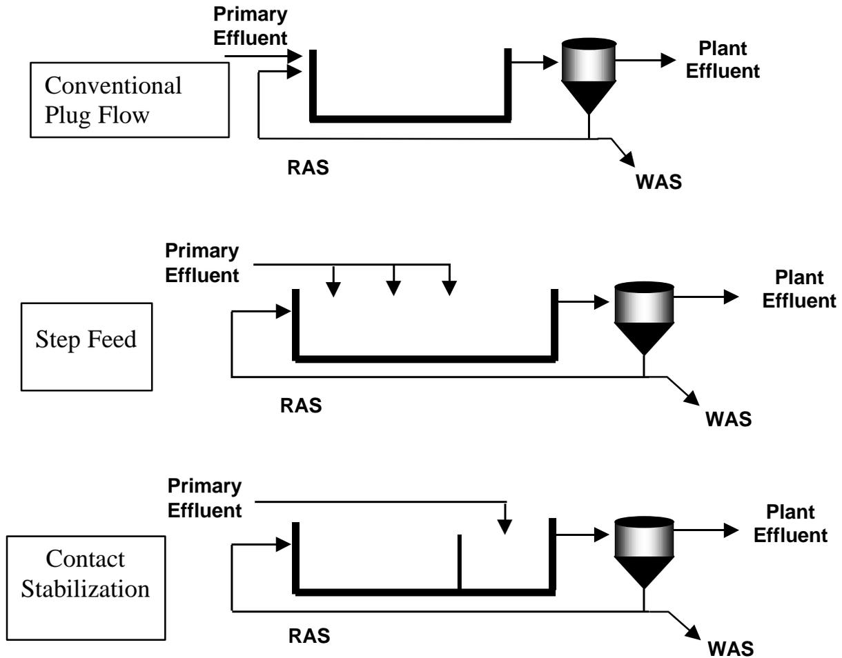
Figure 2.8 Activated Sludge Operating Modes
