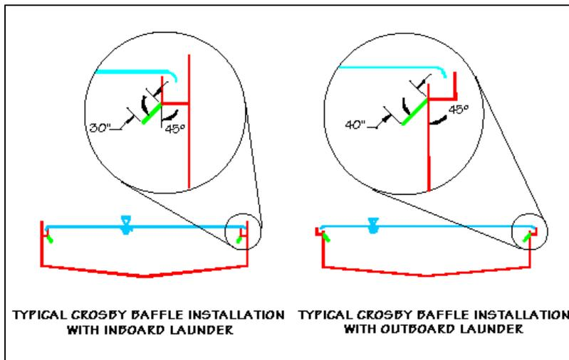
Figure 2.9 Density Current Baffles for Circular Clarifiers
