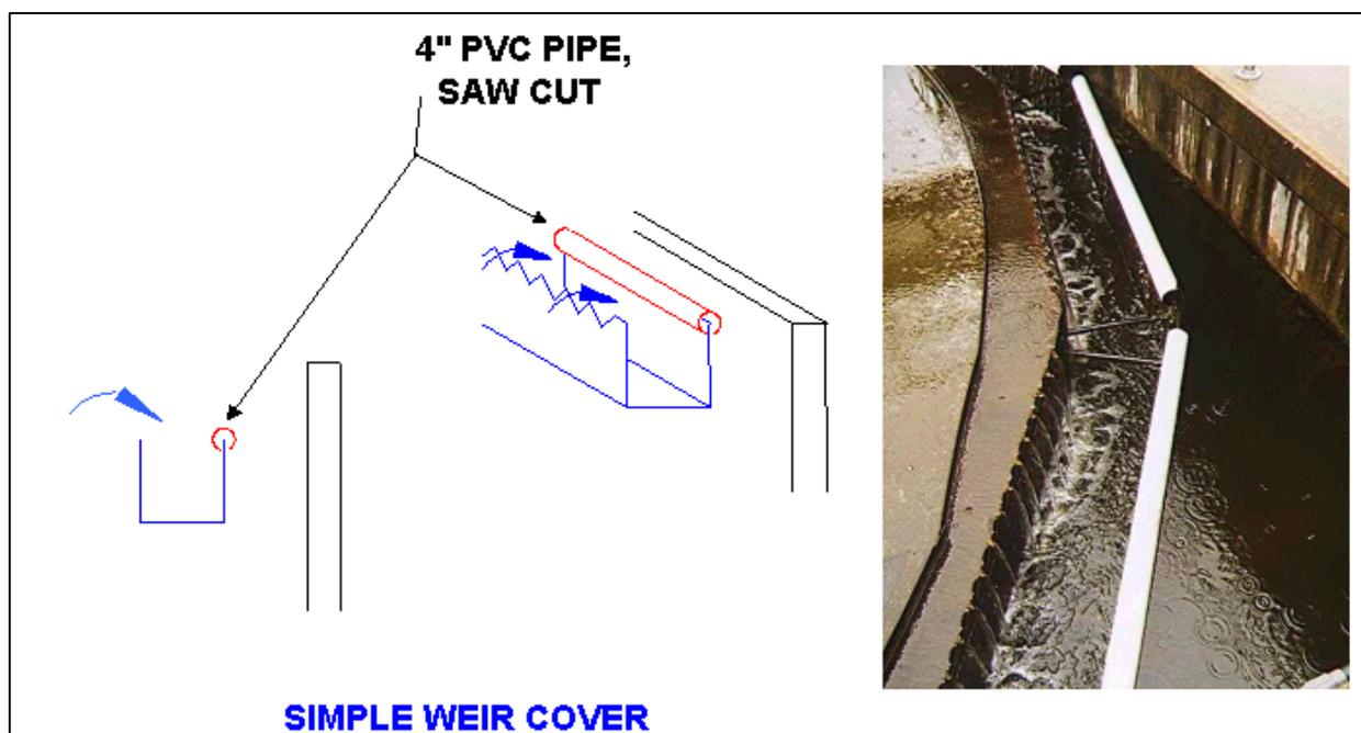
Figure 2.6 Clarifier Weir Block
