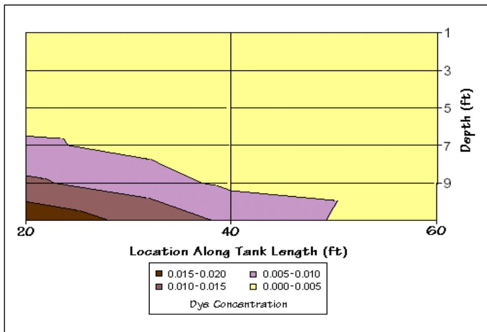
Figure 2.7 Continuous Feed Dye Test at 10 minutes
