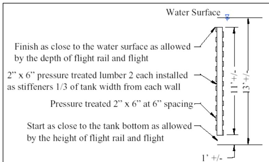
Figure 2.10 Typical Wooden Baffle Construction
