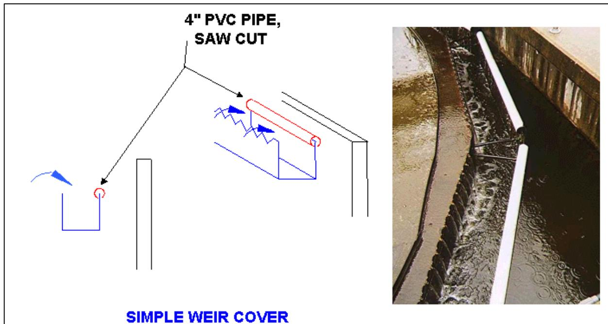
Figure 2.6 Clarifier Weir Block
