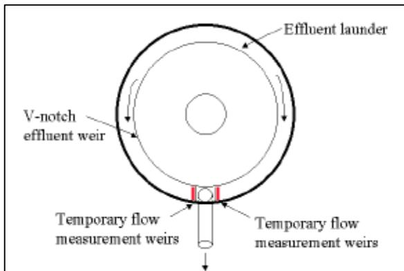
Figure 2.4 Temporary Weirs in Circular Clarifiers
