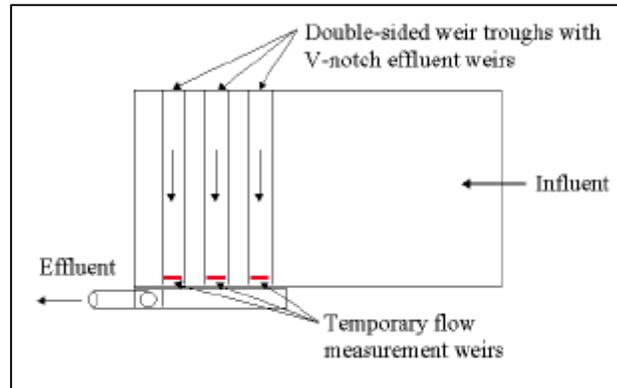
Figure 2.5 Temporary Weirs in Rectangular Clarifiers
