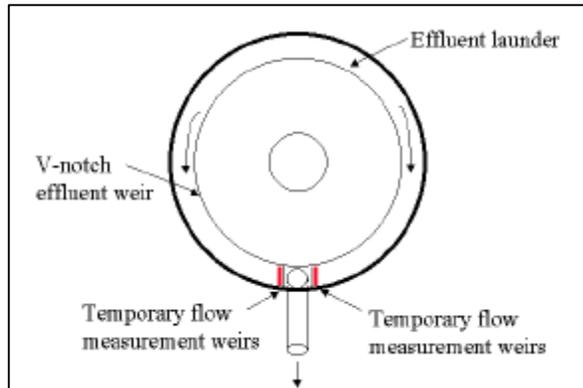
Figure 2.4 Temporary Weirs in Circular Clarifiers
