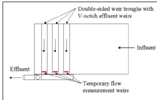
Figure 2.5 Temporary Weirs in Rectangular Clarifiers
