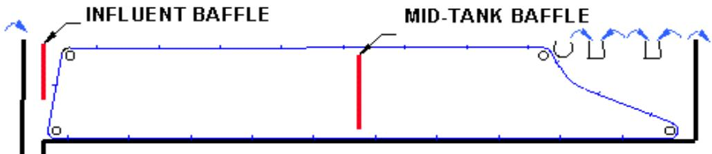
**RECTANGULAR CLARIFIER WITH ONE MID-TANK BAFFLE**
