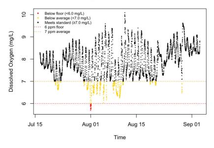
**Figure 9.** Time series of continuous dissolved oxygen measurements in Chenery Brook in 2019.
