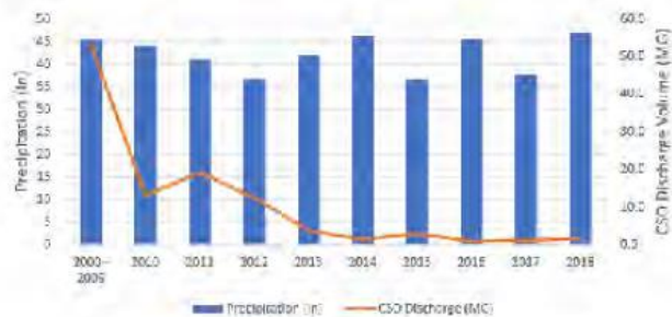
FIGURE 3-6 Auburn Sewer District 2000-2018 Precipitation vs. CSO Discharge
