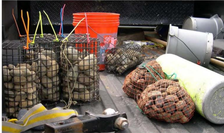
Photo 1. Rock baskets and rock bag samplers before deployment. August, 2021
