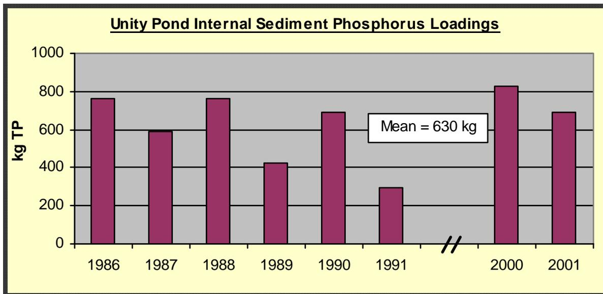
**Linking Pollutant Loading to a Numeric Target:** The basin loading assimilative capacity for Unity Pond was set at 2,060 kg/yr of total phosphorus to meet the numeric water quality target of 15 ppb of total phosphorus. A phosphorus retention model, calibrated to in-lake phosphorus data, was used to link phosphorus loading to numeric target.
