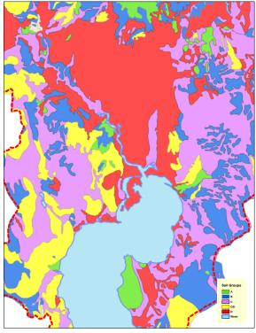
This map displays the hydrologic soil groupings of the northern portion of the Sabattus Pond watershed. The red areas indicate "D" type soils (shown in red) which have the potential for high amounts of runoff.
