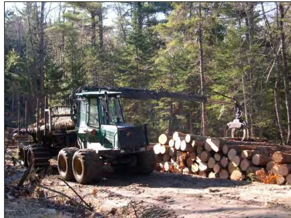
A forwarder purchased with CWSRF-subsidized funding unloading logs.
