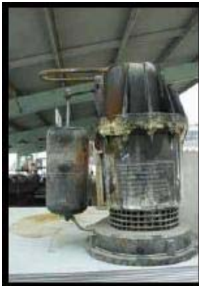
A mercury-free sump pump. Notice the metal guide and no attached wires.
