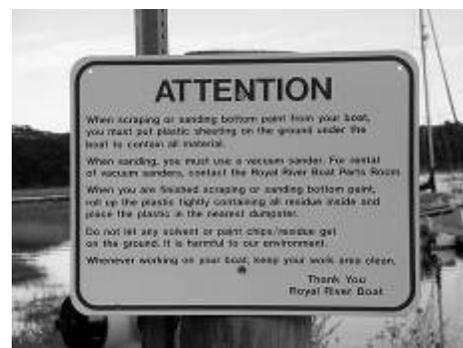
Customer sign on hull preparation. However, the paint debris should NOT be thrown in the dumpster, it should be collected and disposed of as special waste. Photo credit: MEDEP
