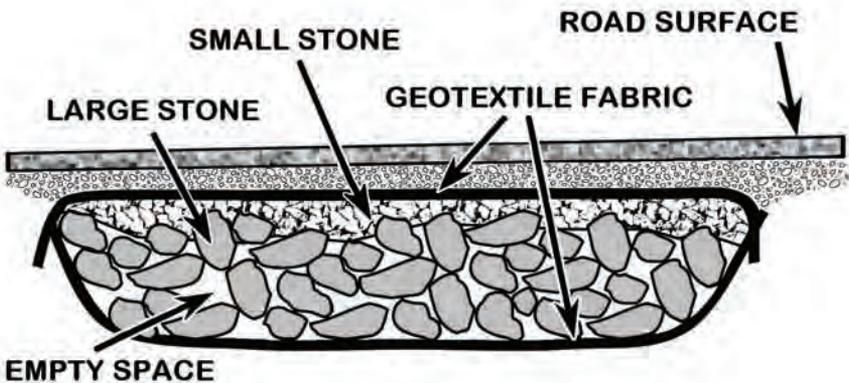
**FRENCH DRAINS** work like a narrow rock sandwich as they are a narrow drainage trench placed parallel to the toe of road cuts with drainage material wrapped in fabric and surrounding a perforated pipe. The drain should be 6 inches in diameter or larger and should daylight to a stable downgradient discharge point.
