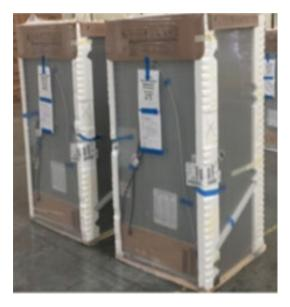
For safety purposes, it is vital to maintain the structural strength of packaging materials, particularly with respect to major appliances that are regularly stacked vertically with multiple units above ground. Furthermore, these appliances are often moved around by clamp truck and the packaging must withstand the force of the clamps to be moved efficiently. Other paper
