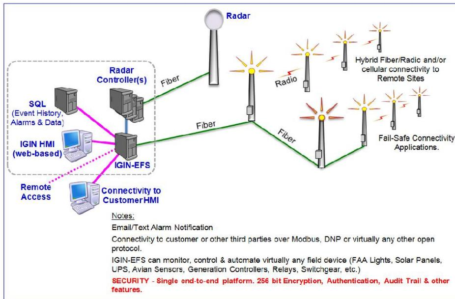
Figure 1: IGIN-EFS example showing typical ADLS components
