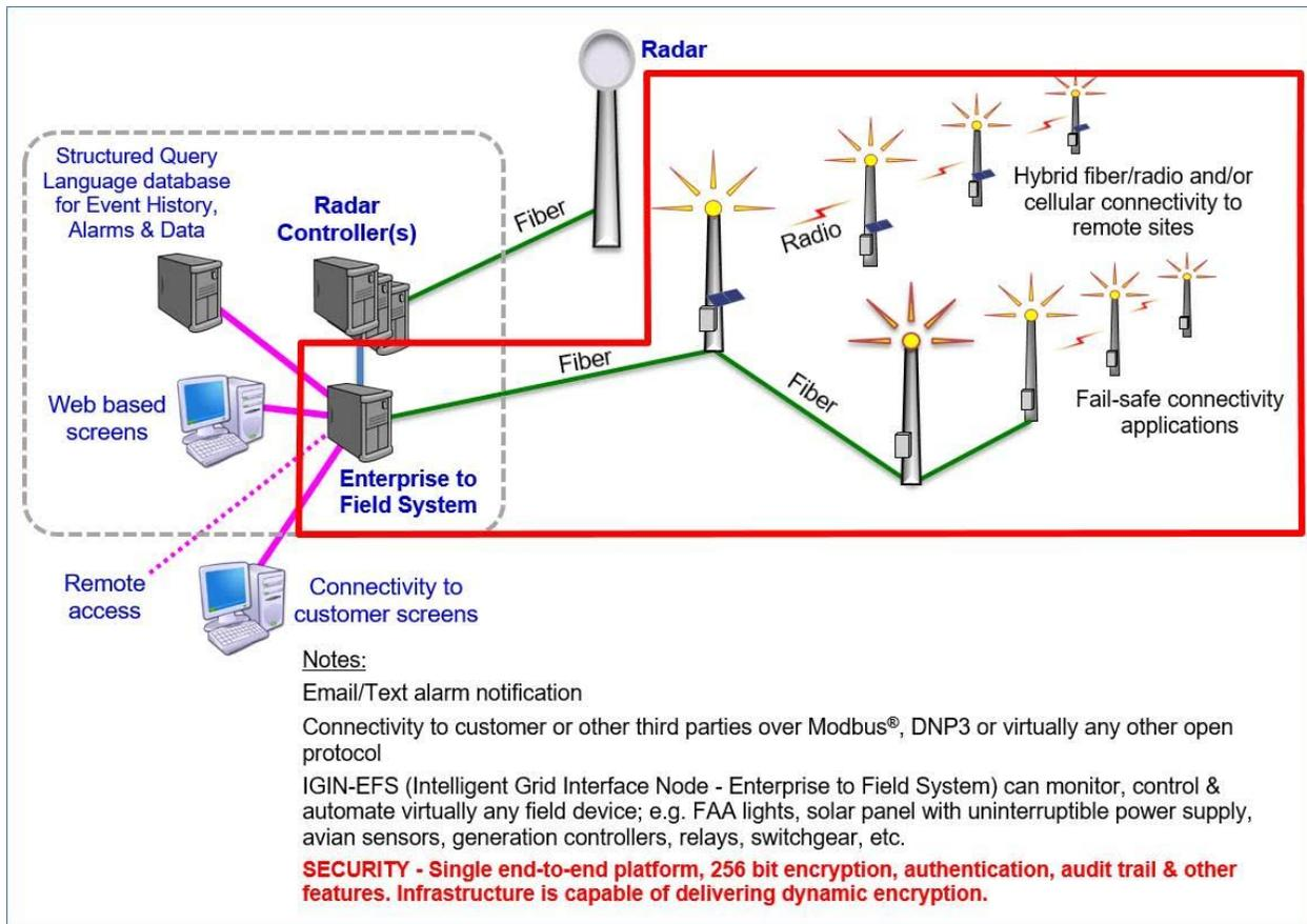
Figure 7. DigitaLogic IGIN-EFS Obstruction Lighting Control System [3]
