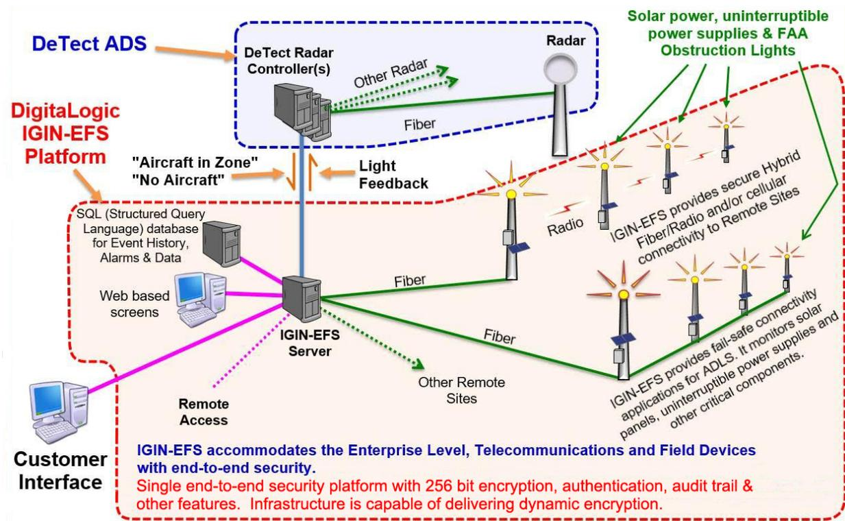
Figure 2. HARRIER ADLS Connected to Other ADLS Components [3]
