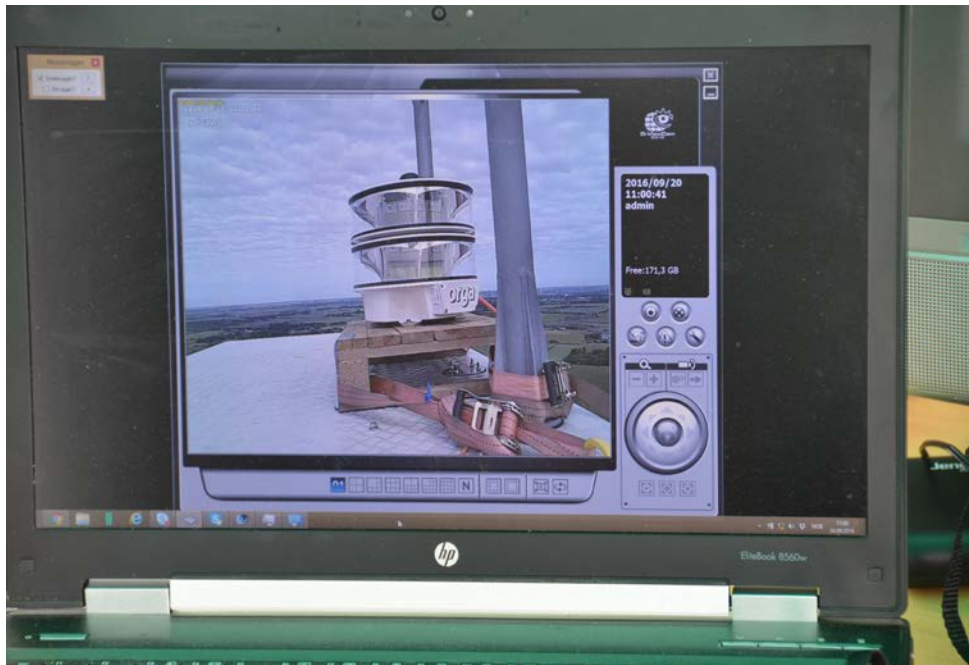
Figure 11. Camera Feed Used to Monitor Obstruction Light Status During Braderup Assessment
