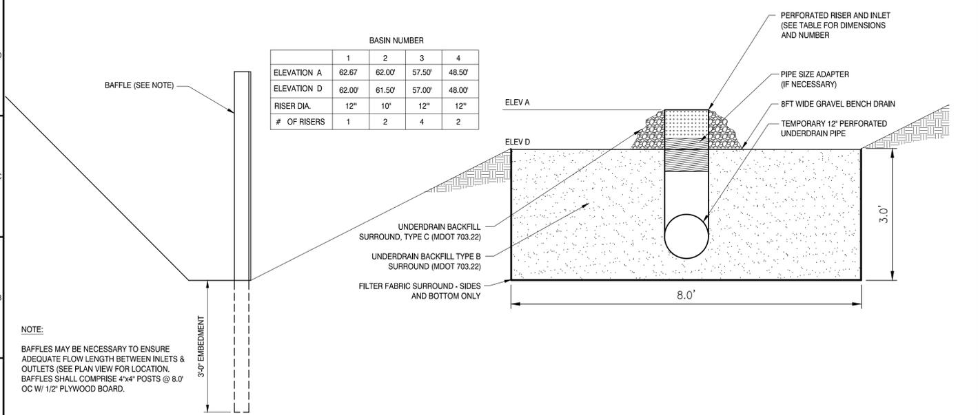
A15 SEDIMENT BASIN GRAVEL BENCH DRAIN OUTLET
