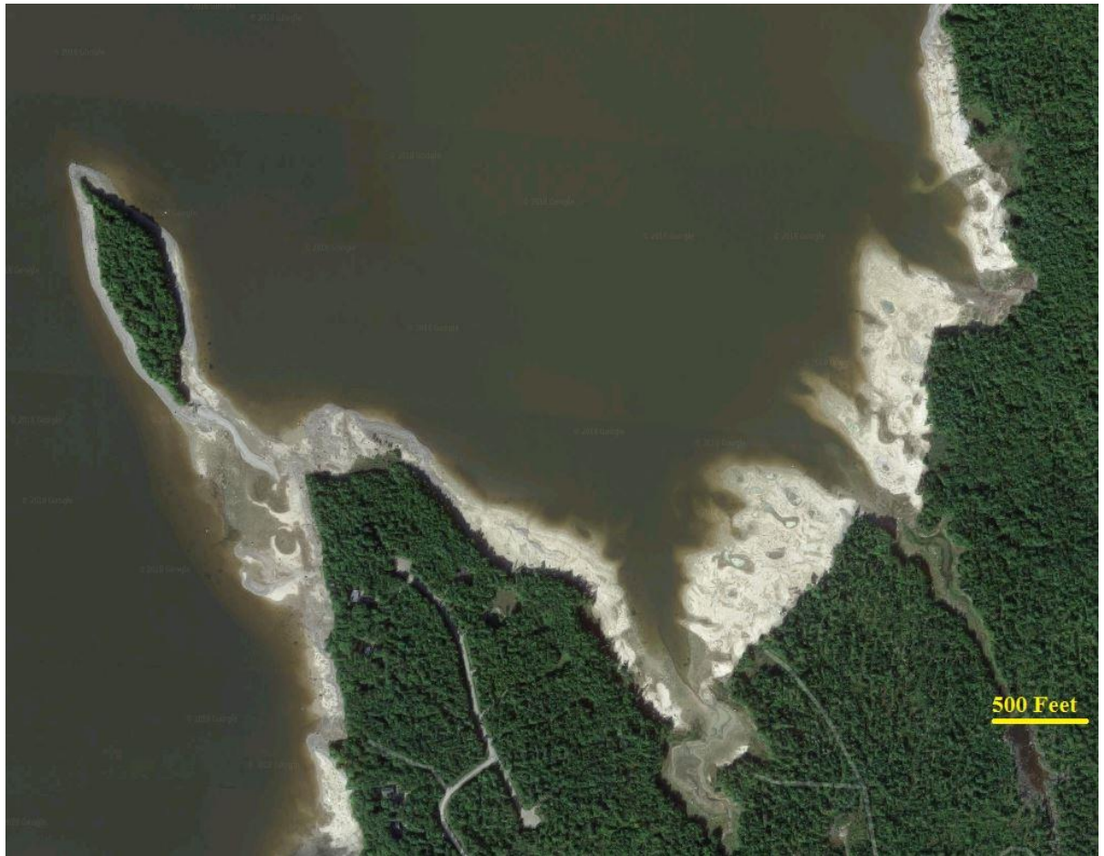
Figure 29. Satellite photograph showing variations in lake bed exposure along the shoreline of Graham Lake on September 25, 2016 (lake elevation at 97.17 feet msl) (Source: Google Earth, as modified by Commission staff).
