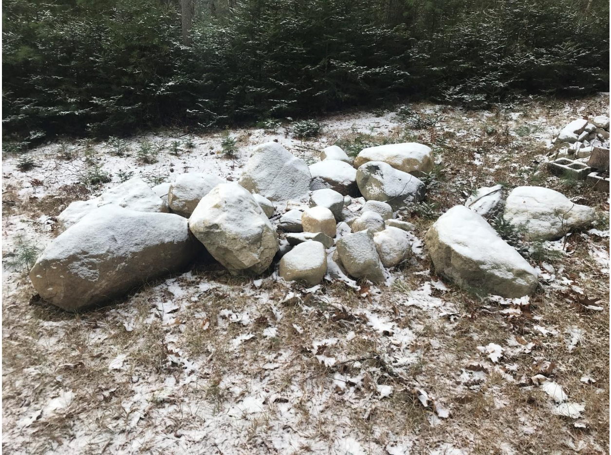
Example of proposed riprap stones; photo sent with email from Jeff Spinney dated 12/4/2019
