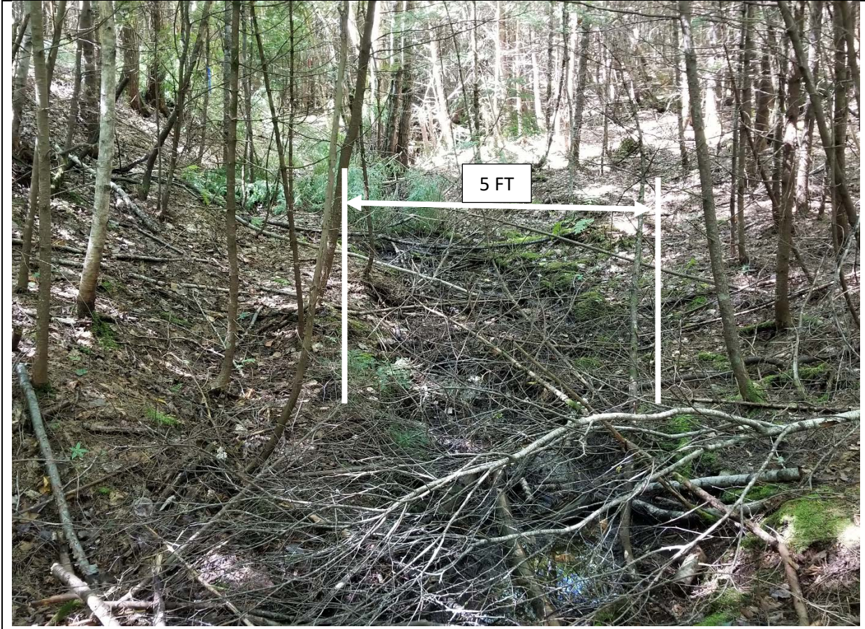
Attachment B: Photo of bankfull width in tributary channel downstream of proposed culvert crossing.
