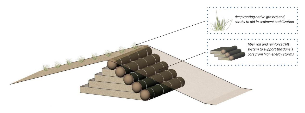
The dune's core contains a reinforced lift and fiber roll system that will help combat wave energy reducing the impacts of erosion during high energy storms. The system is anchored in place, covered by compatible sediment, and planted with a variety of native deep rooting grasses and shrubs to help stabilize the sediment.
