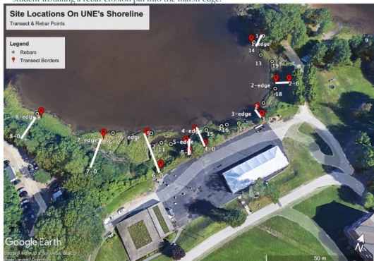
Figure 3. Map of the site featuring each transect and rebar erosion pin location.
