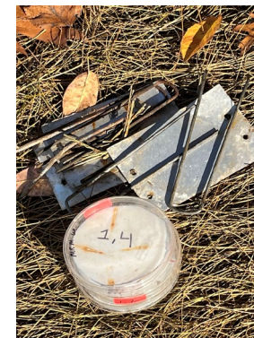
Figure 4. Sediment discs used to measure surface sedimentation rates.
