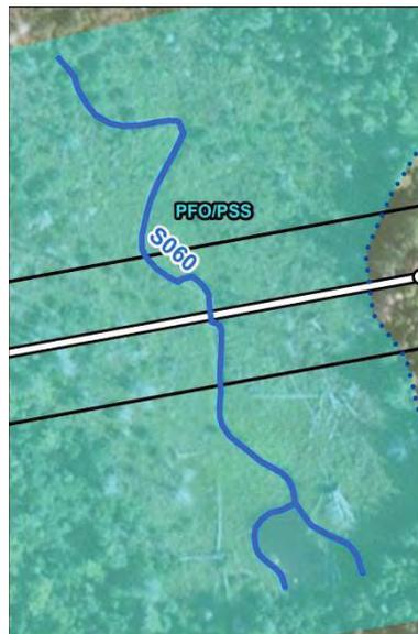
Proposed generator lead crossing of stream S060.
