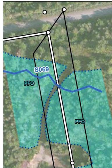
Proposed generator lead crossing of stream S069. Note no proposed impact to wetland ABB\_W384.
