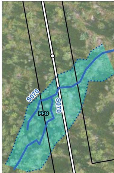
Proposed generator lead crossing of stream S070.
