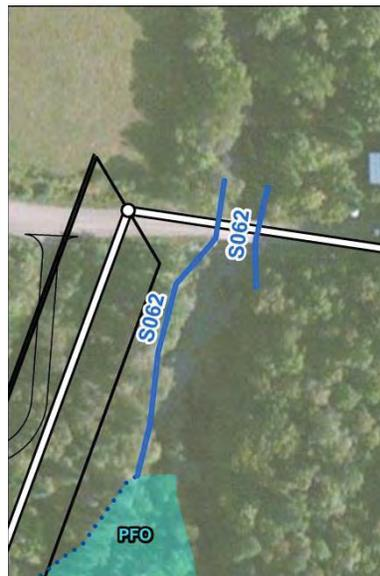
Proposed generator lead crossing of stream S062.
