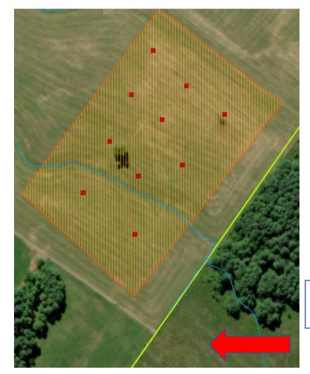
The goal is a representative PFAS value for the Sample Area (orange hash marks). For small fields that will be the entire field (<=10 acres) Sample points should cover the entire sample area, not be biased towards the edges. If there are features such as wetlands and streams sample points should not be placed within the spreading setback around that feature.
