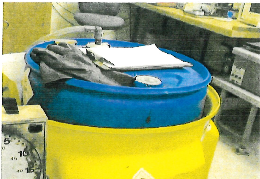
11. Spent waste cyanide and secondary containment vessel, Finish Room.
