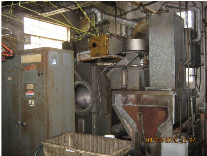
Inoperable dry cleaning machine with vented system.
