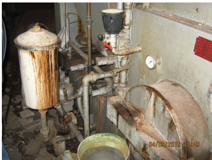
Pre-filter that collects lint and water waste bucket in the back of Renzacci machine.
