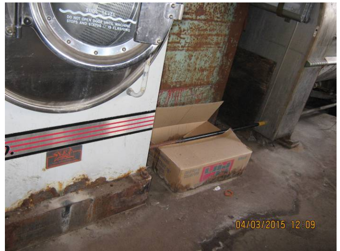
Bottom of Milnor machine and sports equipment painting machine with associated concrete staining.
