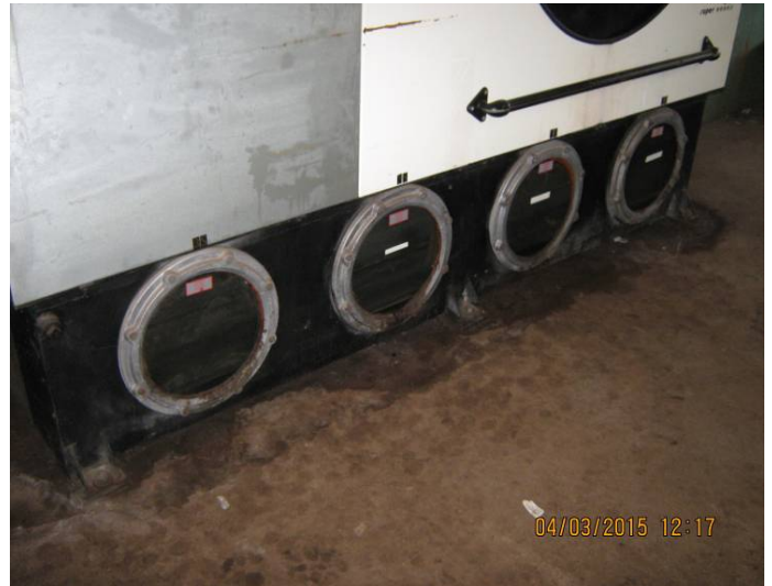
Renzacci dry cleaning machine perc holding tanks and floor staining under machine.
