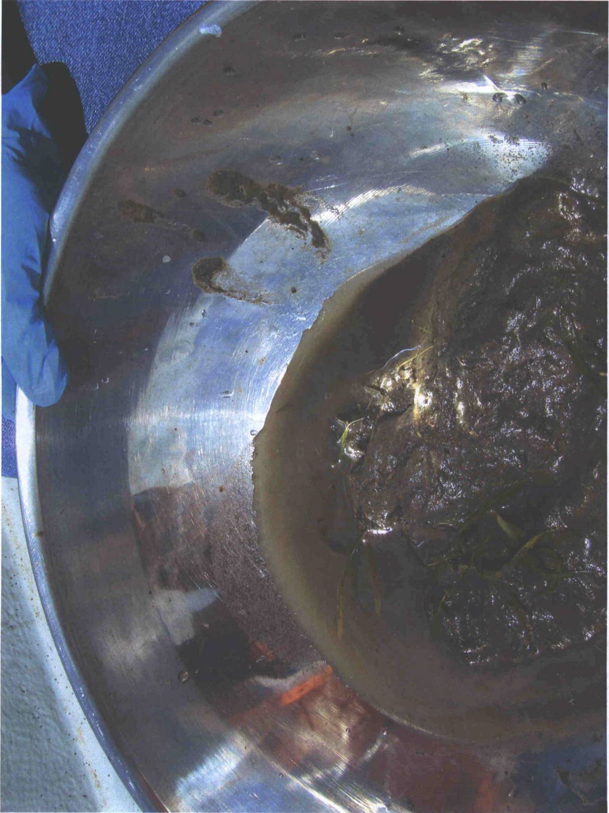
Photograph of weedy silty sediment showing swirl of black oil on water surface.
