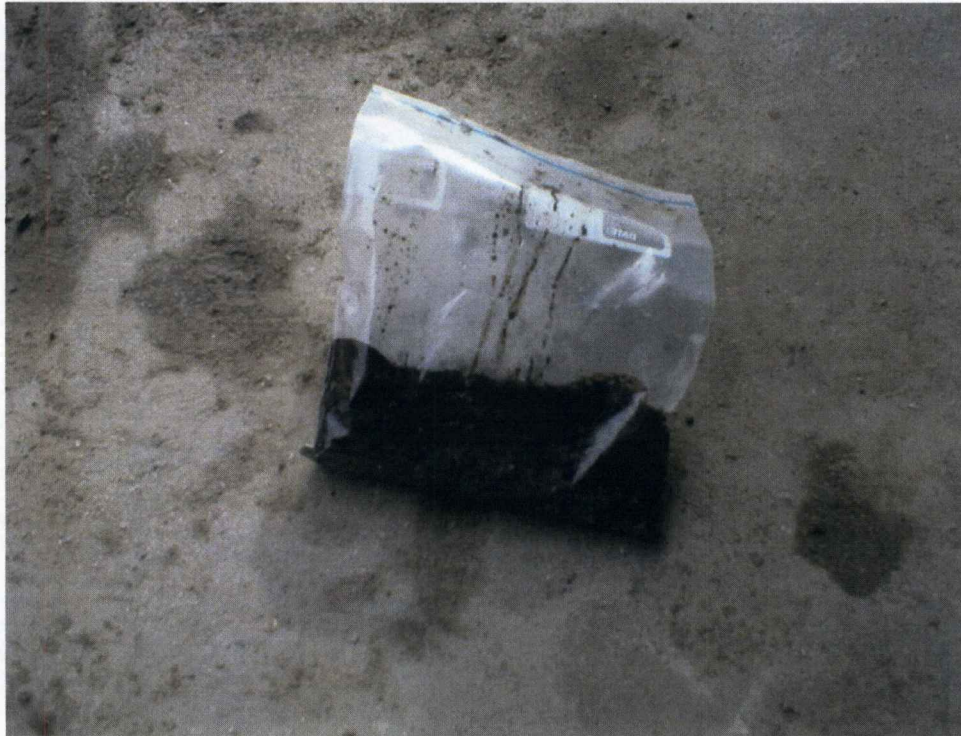
Petroleum saturated soil from boring SB-8
