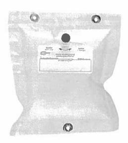
A Tedlar bag is made of two plies of Tedlar film sealed together at the edges and features a valve that allows the interior to be filled. Sample collection requires a pressurized sampling port, a low flow rate pump, or a lung sampler. The bag expands as sample enters. When the target volume of sample is collected, the valve is closed and the Tedlar bag is returned to the laboratory. Air Toxics Ltd. maintains a limited inventory of Tedlar bags in 1 L, 3 L, and 5 L volumes.
