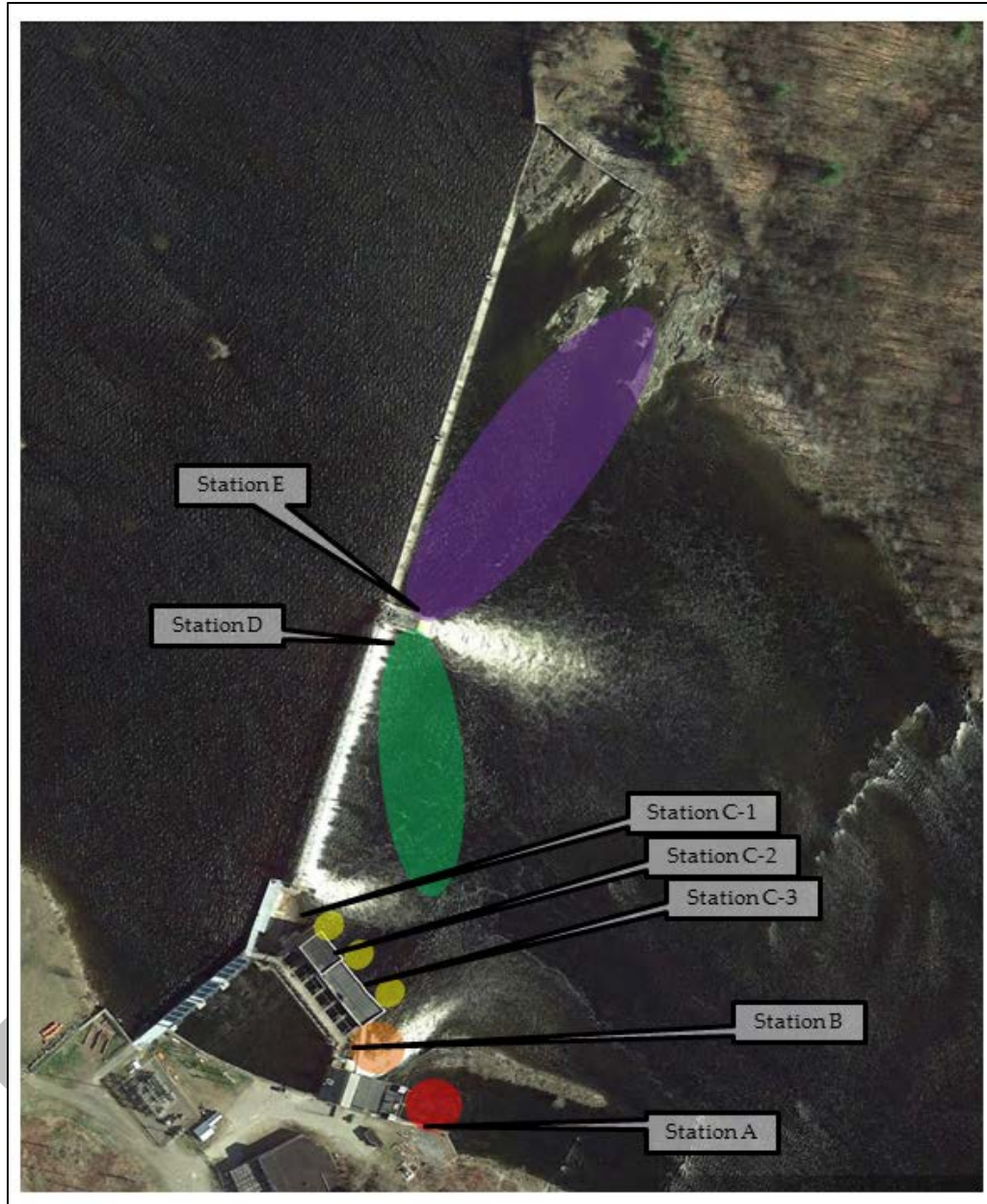
Figure 3-1. Locations of nearfield telemetry monitoring stations A through E at Shawmut, Kennebec River, Maine, May-June 2016.
