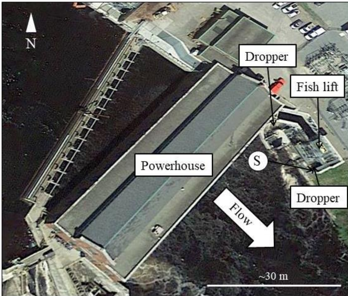
Figure 2.2. Aerial view of the Milford Dam powerhouse on the east side of the river showing the locations of the two dropper antennas relative to the fish lift. The S indicates the position of the stationary radio receiver and associated Yagi antenna.
