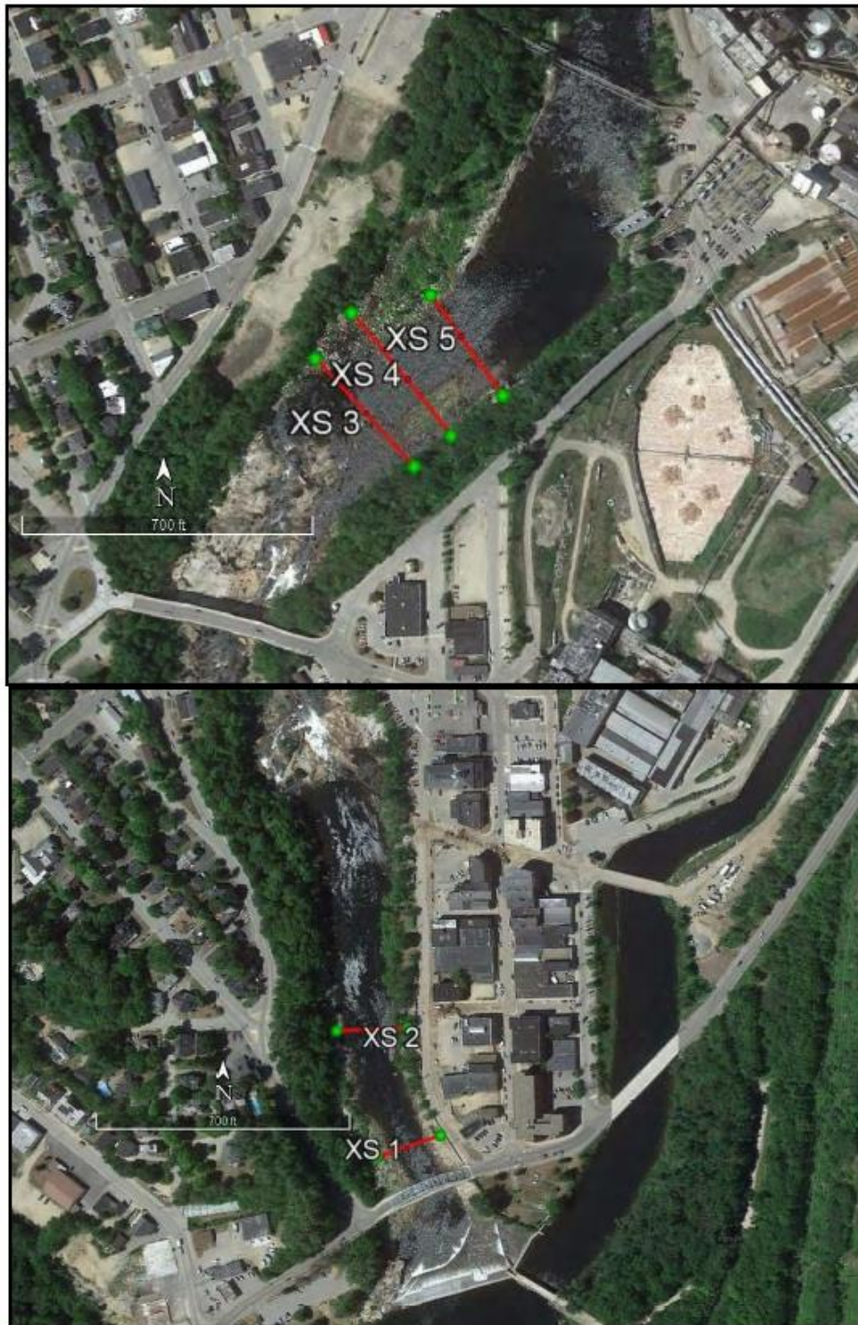
FIGURE 5.6-3 MIDDLE DAM BYPASS REACH CROSS SECTIONAL TRANSECTS 1 AND 2 IN THE UPSTREAM END OF THE REACH (BOTTOM IMAGE) AND 3, 4, 5 IN THE DOWNSTREAM END OF THE REACH (TOP IMAGE)
