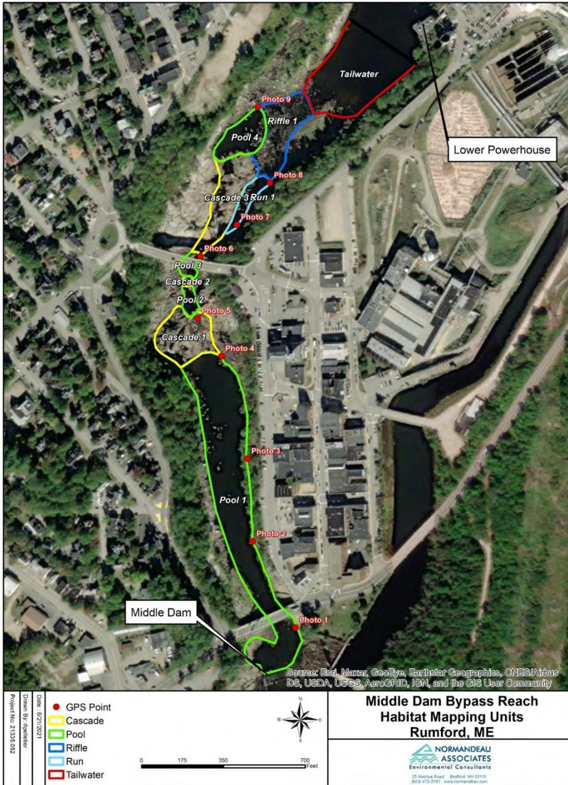
FIGURE 5.6-2 MIDDLE DAM BYPASS REACH HABITAT MAP UNITS AS CHARACTERIZED DURING MESOHABITAT MAPPING ON JUNE 8, 2021 (RFH 2022)
