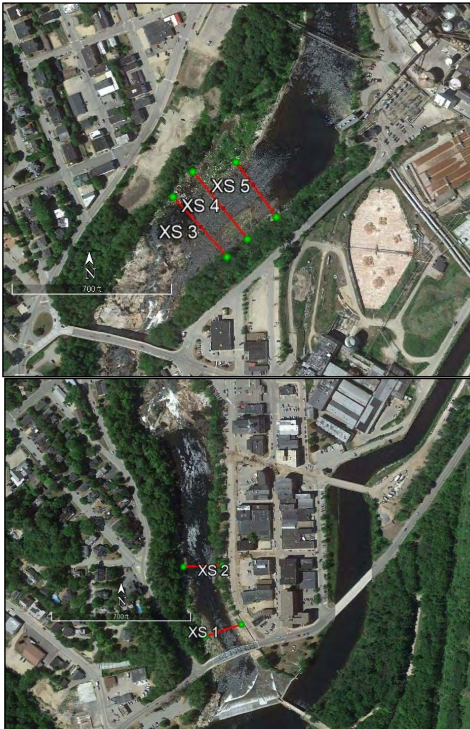
Figure 2 Middle Dam bypass reach cross-sectional transects 1 and 2 in the upstream end of the reach (bottom image) and 3, 4, and 5 in the downstream end of the reach (top image)
