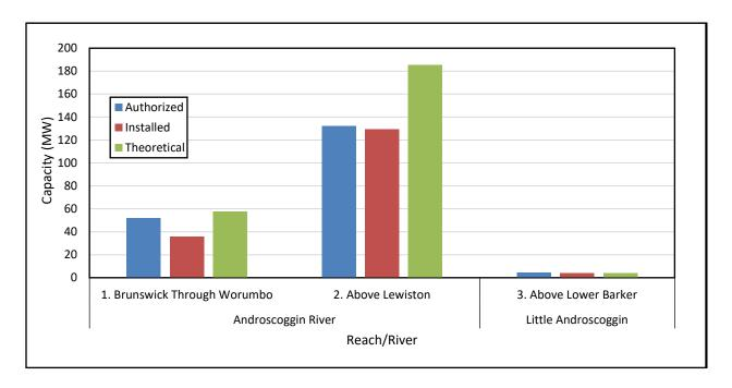
Figure 18. Summed capacities for FERC licensed project. Authorized represents the capacity of the FERC license. Installed is the capacity that is currently available. Theoretical is based on the methods described in Section 8.
