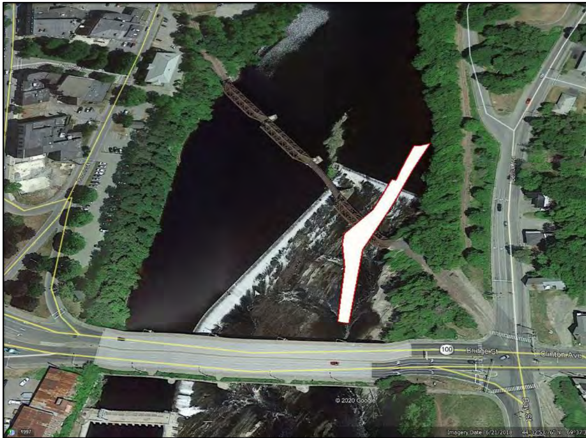
PHOTO 1 APPROXIMATE PROPOSED FISH LADDER PLACEMENT, ALONG THE EAST SIDE OF THE KENNEBEC RIVER, UNDER THE RAILROAD BRIDGE, OVER THE NORTH SECTION OF THE DAM
