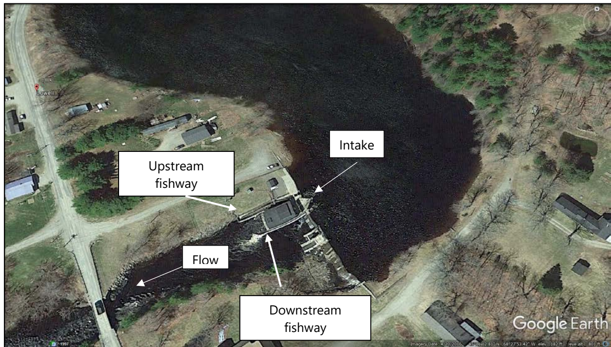
Photo 2.2 Aerial Imagery Showing Location of Upstream and Downstream Fishways and Angled Intake Racks at the Lowell Tannery Project.
