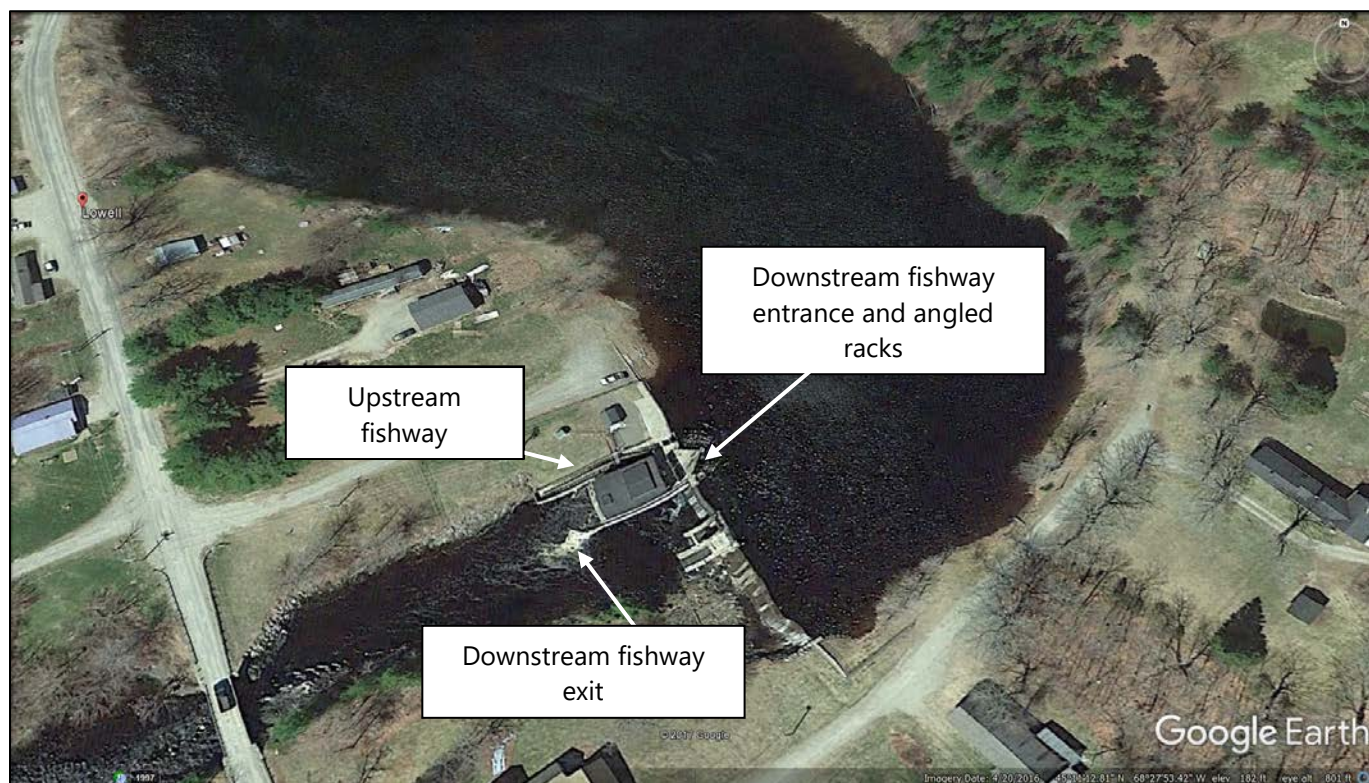
Photo 4.4 Aerial imagery showing location of upstream fishway, downstream fishway, and angled intake racks at Lowell Tannery Project.
