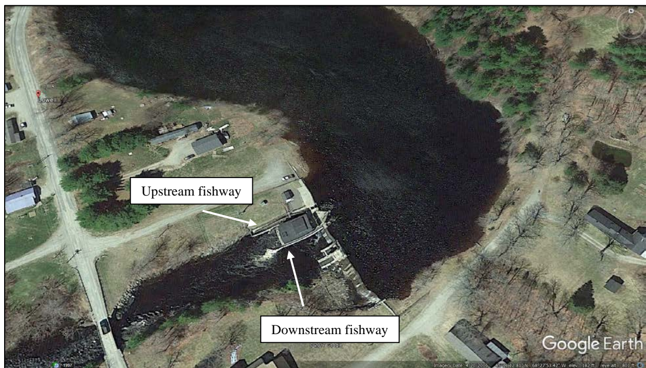
PHOTO 1. AERIAL IMAGERY SHOWING LOCATION OF UPSTREAM AND DOWNSTREAM FISHWAYS, ANGLED INTAKE RACKS, AND POWER CANAL AT THE PUMPKIN HILL PROJECT.
