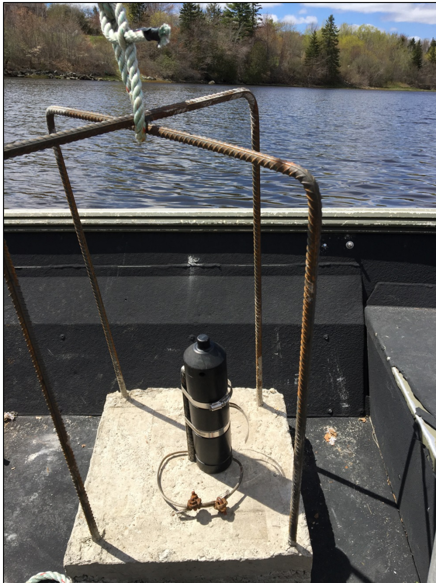
Figure 2-2. Vemco VR2W acoustic receiver and mooring platform deployed in the Union River during the 2017 downstream smolt passage evaluation.
