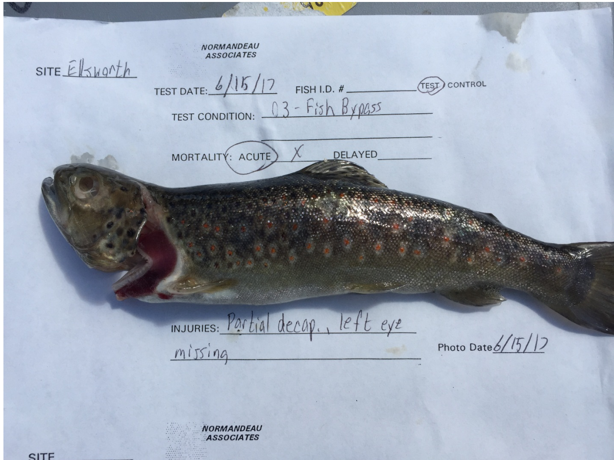
Figure 4.5. Single recorded major injury sustained by an individual fish released through the downstream bypass.
