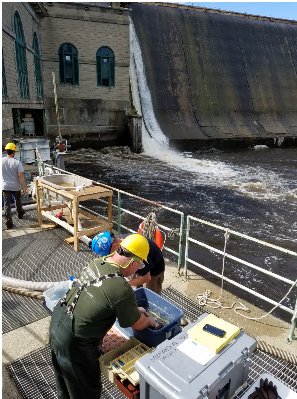
Figure 3.3. Fish tagging site with induction system at left. The release basin sat atop a wooden frame with the release pipe below. This was the control release system, and an identical system was used to release treatment fish into each passage route.
