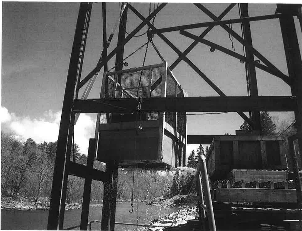
Photo 3. The hopper capacity does not include the screened wall panels. The capacity is only based upon the watered up portion of the hopper as measured from the interior walls. Photo: Don Dow, NMFS.
