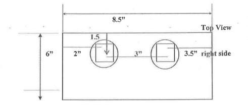
Counter sunk holes Holes are 1 ½" FROM TOP Size; 5/8"x 6" x 8.5" Blade Steel Plate to make curb shoes
