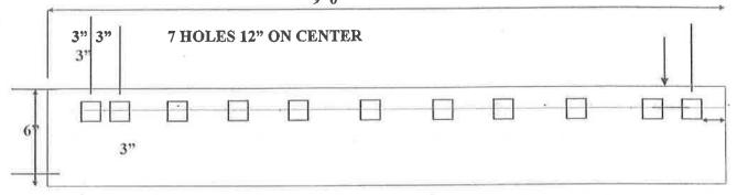
SIZE: 3/4" X 6" X 108" All holes to be punched 11 holes 11/16" sq. Spaced as shown above. Plow Blade 3/4" thick From left to right first two (2) are 3" apart on center, and then the next 7 holes are 12" on center, then 3" on center, then 3" on center
