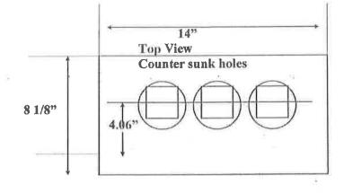
Size; 1" x 14" x 8 1/8" Blade Double Bevel Flat Bolt Size = 3/4" x 2 3/4"
