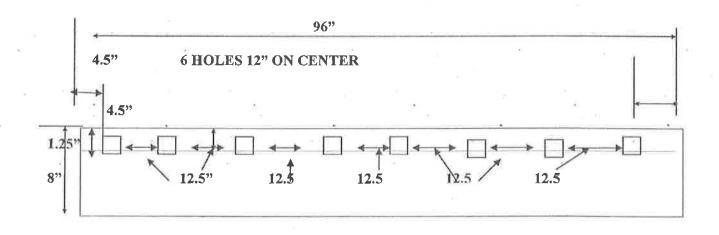
SIZE: 5/8" X 8" X 96" All holes to be punched 6 holes 11/16" sq. Spaced as shown above. Plow Blade 5/8" thick From left to right first hole is 4.5" apart on center, and then the next 6 holes are
