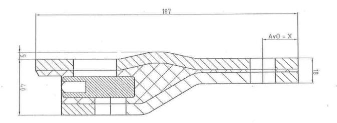
Figure 2: AASHTO Hole Positioning (4')
