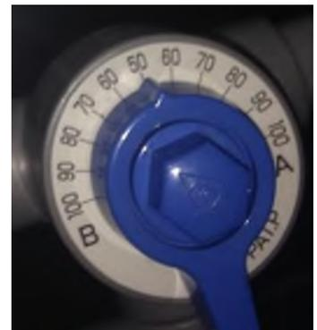
At start-up, and for standard operation, the Aeration Balance Control Valve (blue) should be set to 50%,
