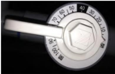
**B.** Transfer the sludge on the bottom of the aeration chamber by turning the Recirculation Control Valve (grey valve) to 70-80 and wait for one minute.
