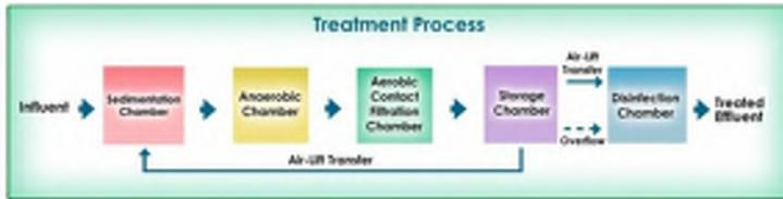
**Two Air Lift Pumps.** One Recirculating Air Lift pump sending process water and solids back to Chamber 1, and one Effluent Air Lift Pump for measured discharge of treated effluent. (See airlift pump info below).
