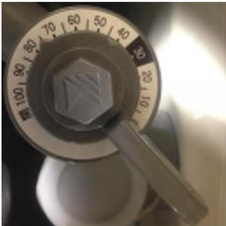
**C.** Reset the Recirculation Control Valve (grey valve) to the original position.
