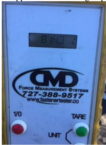
Pull test #1 as test passed 805lbs = 195PSF Test was stopped after exceeding requirements
