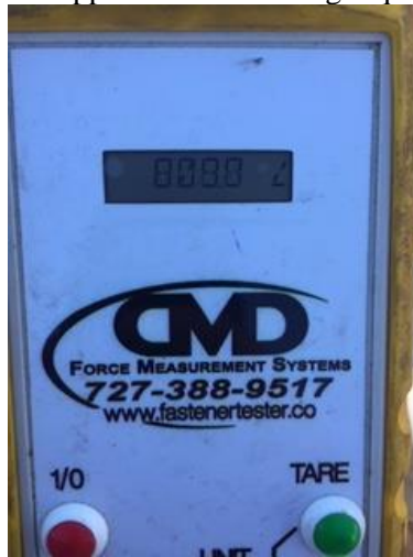
Pull test #2 as test passed 805lbs = 195PSF Test was stopped after exceeding requirements
