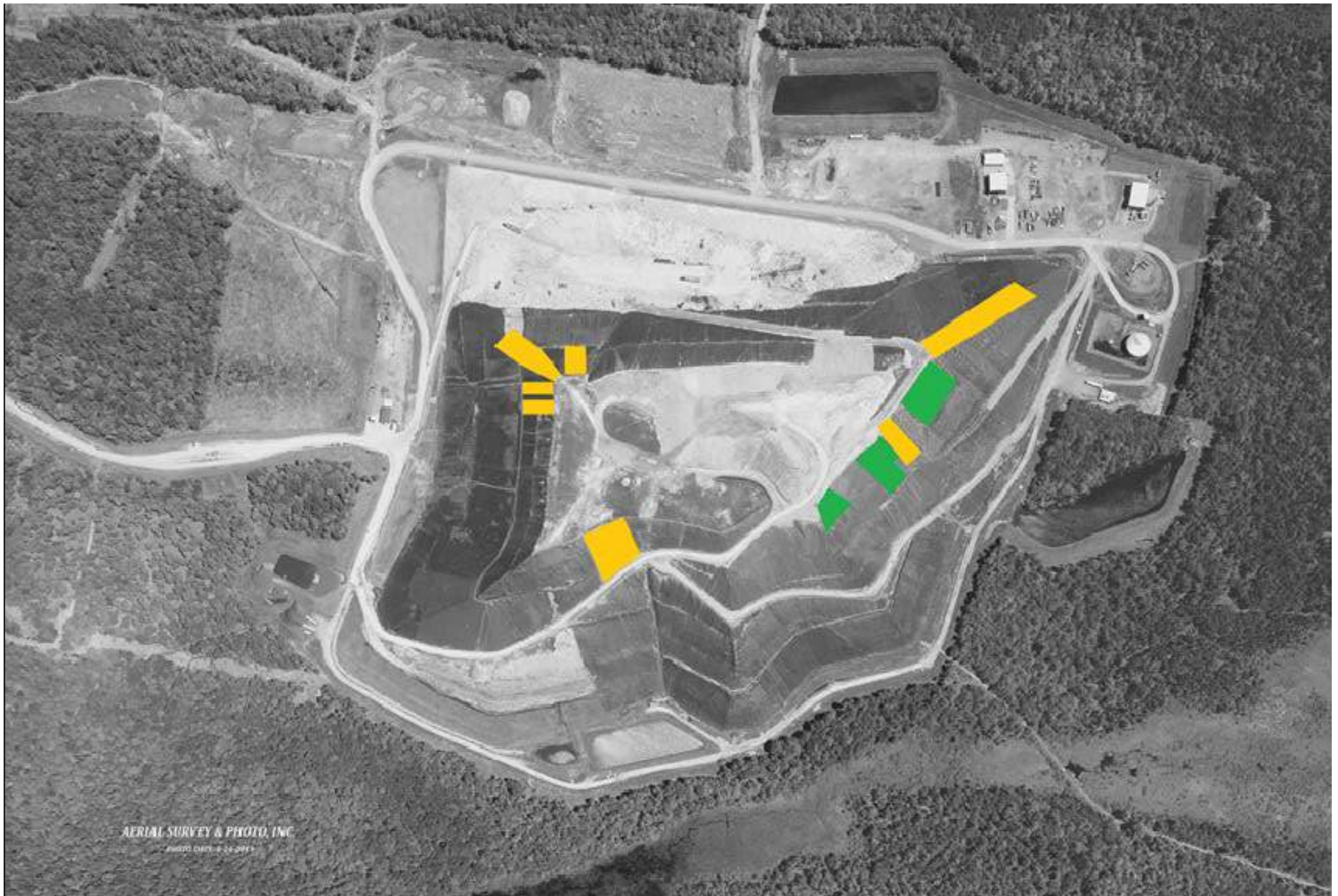
Key: Sand Ballast (yellow); Platypus Anchors (Green)
