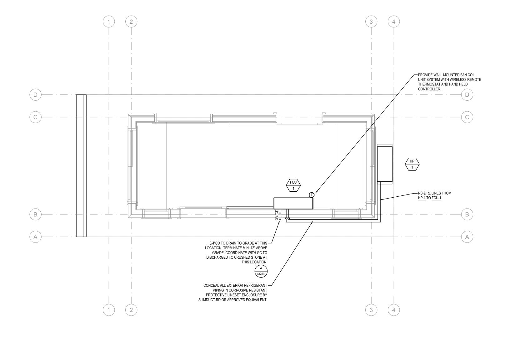
1) MECHANICAL GATEHOUSE FLOOR PLAN SCALE: 1/2" = 1'-0" MECHANICAL PLAN NOTES:
