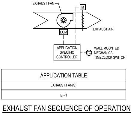
THE EXHAUST FANS SHALL BE CONTROLLED THROUGH THE APPLICATION SPECIFIC CONTROLLER AND THE WALL MOUNTED DIGITAL TIMECLOCK SWITCH. THE SEQUENCE LISTED BELOW IS REVERSIBLE UNLESS NOTED OTHERWISE.
